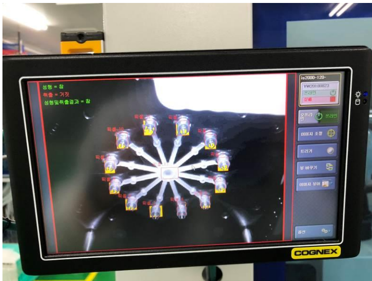
Fig. 3a: Quality inspection of sealing caps (Photos: Wittmann Battenfeld)
