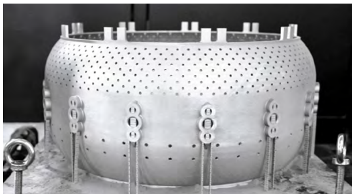
High Temperature Alloy Combustion Chamber
